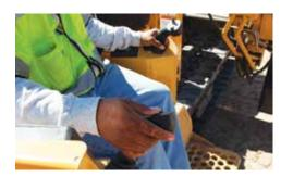
TAKE CONTROL. Conveniently placed dual joystick controls allow the operator to control machine functions including engagement of the hammer, pile placement and ground drive.
